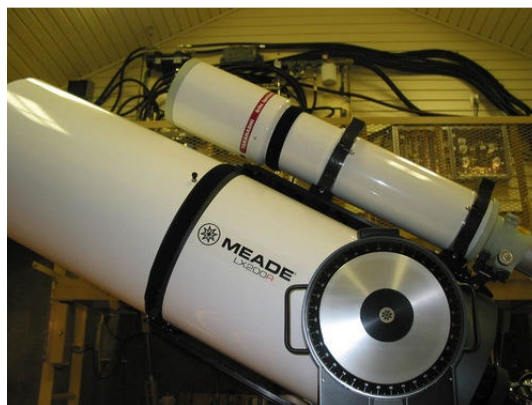
Figure 2. The two primary telescopes of the observatory – a Takahashi TOA 150 piggybacked on the Meade 16" Ritchey-Chretien telescope.
