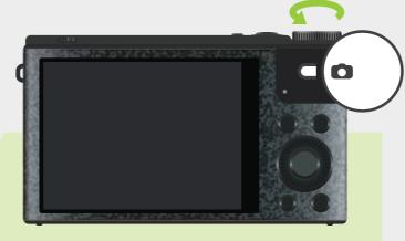
2 Rotate the Mode Dial to AUTO. Align the icon with the marker.
