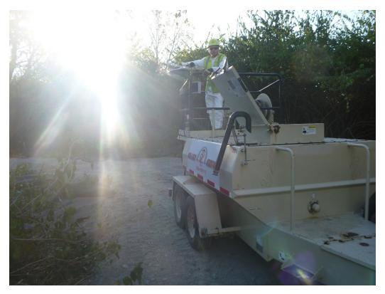
The photo was taken outside the OU1 area, the view is facing west. The photo shows the air monitoring system being used to measure/detect any off-site release at the fence line. The "system" consists of a TLD, Alpha Track Radon detector and a particulate filter. This is 1 of 13 monitors in/around the perimeter of the WLLS.
