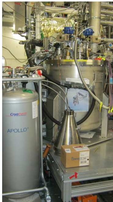
Fig. 33 – A CSC at GSI: the gold-colored cylinder in the upper side of the figure. The cryogenic unit is in the center and its precooling Dewar vessel is on the left side. Published with permission of GSI.
