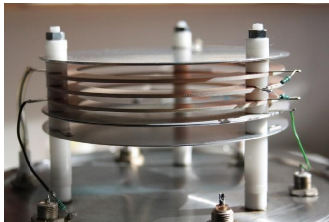
Fig. 16 – Photograph of the one-sided BIC used for the present test measurements.
