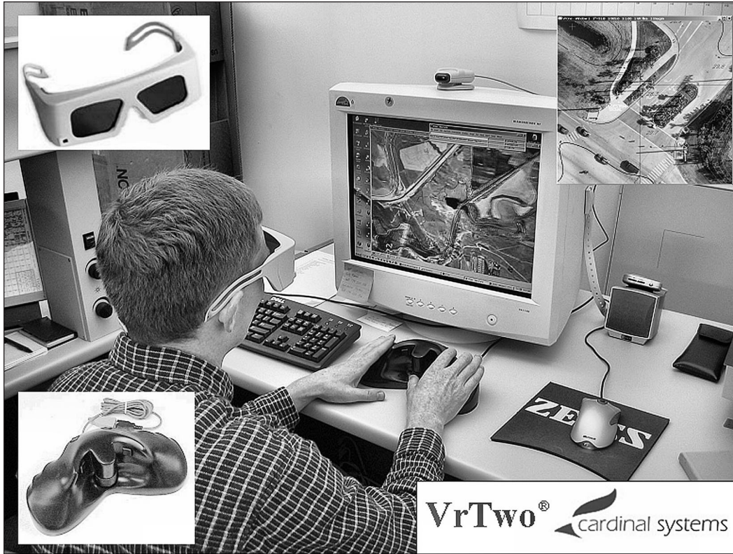
Figure 8. Digital or “soft copy” photogrammetry workstation using VrTwo software, showing stereo glasses and “3-D mouse”.
