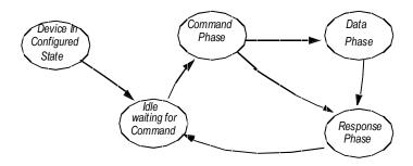
Figure D.3: Operation Phase State Diagram
