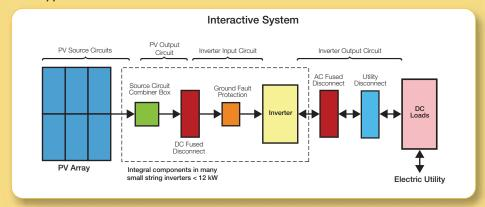
inverters can provide stand-alone power for critical loads independent from the grid during outages. See Figure 16.
