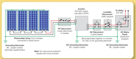
Electrical resistance and continuity testing can be used to confirm the following NEC requirements:
