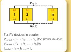
Figure 12. Connecting similar PV devices in parallel increases current while voltage stays the same.
