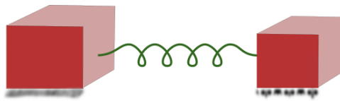
Figure 2: Two masses separated by an actuator that can change its length. If the two masses have bases with different frictional coefficients and the actuator's length varies periodically but not sinusoidally, then the scallop can inch forward. A model explored by Wagner and Lauga 2013.
