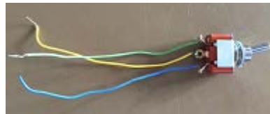
SPDT switch has 3 terminals
