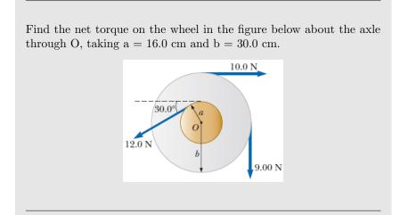
A torque that's produced by a force can be calculated from the expression:  $\tau = F \cdot r \cdot \sin \theta$ . All the forces acting on the wheel are perpendicular to the rotation axis with  $\theta = 90^{\circ}$  (the 30° is irrelevant in this picture). By taking the clockwise direction as positive, We should have:
