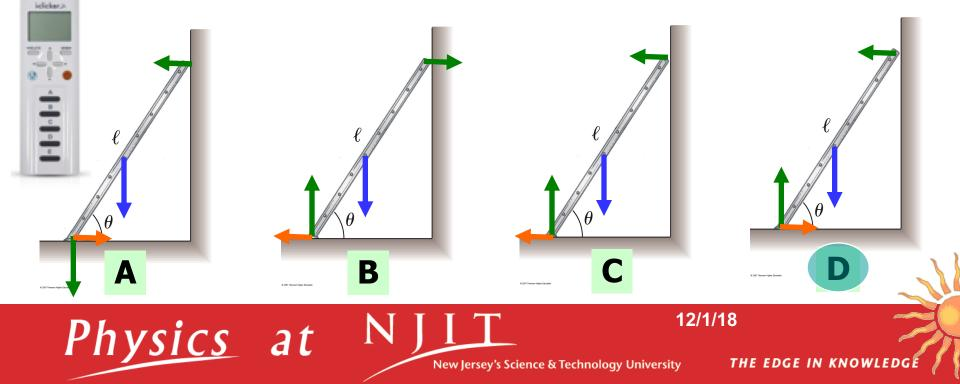
□ A uniform ladder of length *l* rests against a smooth, vertical wall. The mass of the ladder is m, and the coefficient of static friction between the ladder and the ground is  $\mu_s = 0.40$ . Find the minimum angle  $\theta$  at which the ladder does not slip.
