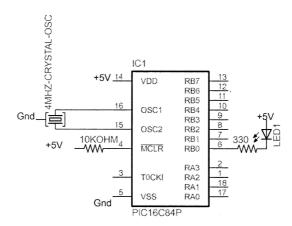
The remaining pins can remain unconnected for now. We will turn the LED on and off by changing the value output at pin PortB.0. Will the LED be lit when the value is High or Low?
