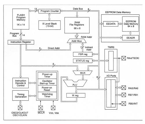
Note that things are slightly more complicated than the simple diagram above would indicate. But the essentials are the same. You should roughly consider the Flash Program Memory to correspond to the Program Memory in a simplified Harvard Processor and the RAM File Registers and EE Data Memory to correspond to the data memory. To jog your memory on Harvard Architecture computers and memory, review your class lecture notes.
