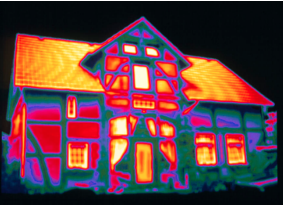
Thermogram showing heat loss from a house.
