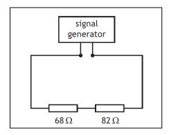
Determine the r.m.s. voltage across the 82  $\Omega$  resistor.
