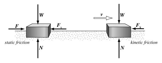
*Example 3.* A 24 kg crate is moving at a constant velocity along a horizontal floor because of a 75 N horizontal force pushing it along.
