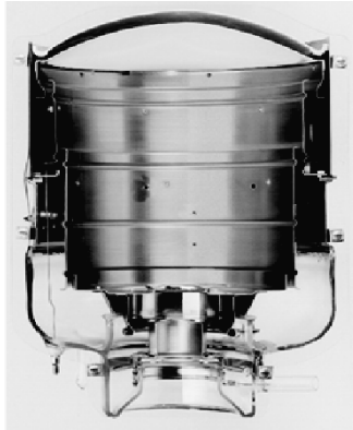
classical RII made of glass. Notice the glass cover, the electrode system made of steel, the primary screen at the upper part, and the secondary screen at the lower part
