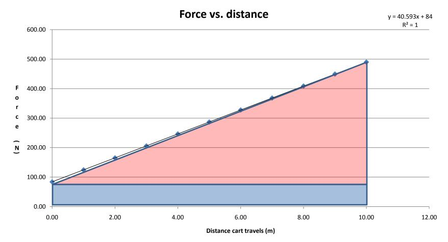
Work = Force x distance but also is the area under the curve. Area of rectangle + area of triangle.  $\sim$ 100N x10m + 1/2x $\sim$ 500Nx10m = 3500N
