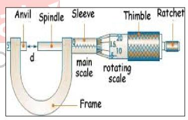
The smaller stud is known as the anvil and the longer one is known as the spindle. The anvil is fixed part of device, whereas the spindle moves. The object to be measured is held between the anvil and the spindle.
