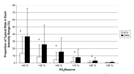
FIGURE 4—The cumulative proportion of a recreational trail ride in each exercise intensity range ( $\%\dot{V}O_2R$ ) and by vehicle type. \*Significantly different proportion of ride spent at a given intensity between ATV and ORM, P < 0.05.
