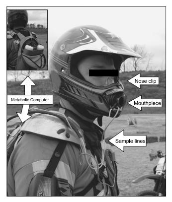
FIGURE 1—Ambulatory oxygen consumption measurement while riding an off-road vehicle. The rider's nose is plugged and all expired air is expelled through the mouthpiece which contains a volume meter and expired air sample line held in place by the modified chin guard of the helmet. *Inset top left:* Reverse angle view of the metabolic computer (with protective padding) in the backpack as worn by riders.
