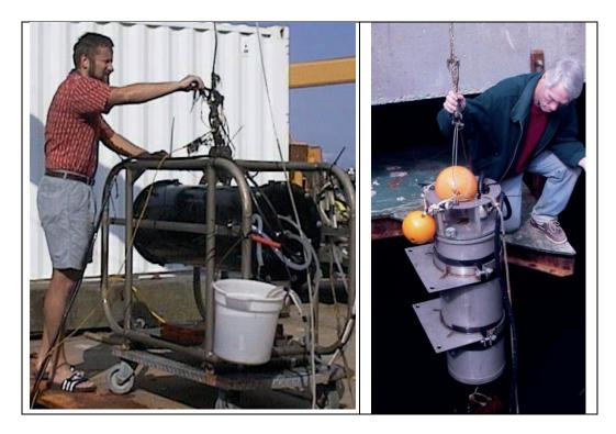
Figure 3. FlowCytobot (left) and Imaging FlowCytobot (right) ready for underwater deployment in their pressure housings and mounting frames.
