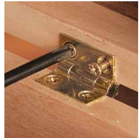
Mortises for butt hinges. The router table makes quick and accurate work of removing the majority of the waste. The corners can be squared up with a chisel before installing the hinge.
