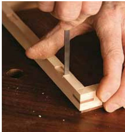
Mortises for butt hinges. The router table makes quick and accurate work of removing the majority of the waste. The corners can be squared up with a chisel before installing the hinge.
