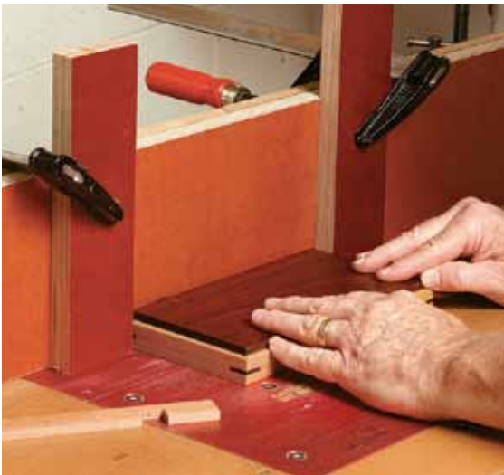
Mortises for butt hinges. The router table makes quick and accurate work of removing the majority of the waste. The corners can be squared up with a chisel before installing the hinge.
