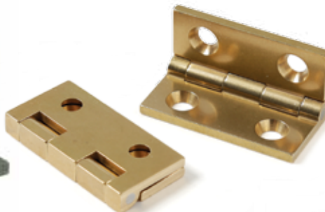
Blocky in the back. Most stopped butt hinges have a squared-off knuckle, as compared to the rounded knuckles of the non-stopped varieties.
