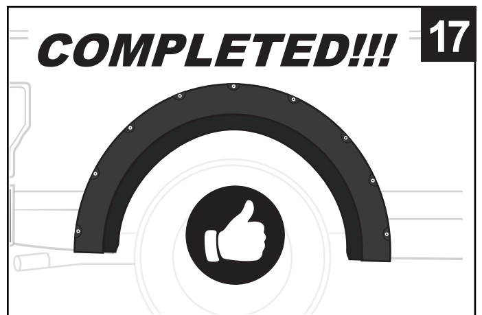
17. Tighten all 5 screws from STEPS 14-15 to complete installation. Repeat STEPS 8-17 to the other side.
