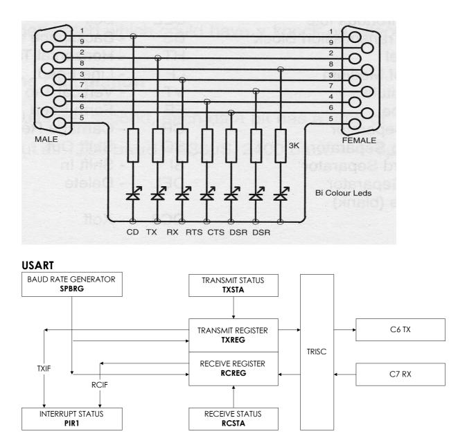
The USART operates in one of three modes: Synchronous Master, Synchronous Slave and Asynchronous, the latter being the most common for interfacing peripherals. Besides the obvious interface to PC's and Modems, the USART can interface to A/D, D/A and EEPROM devices.
