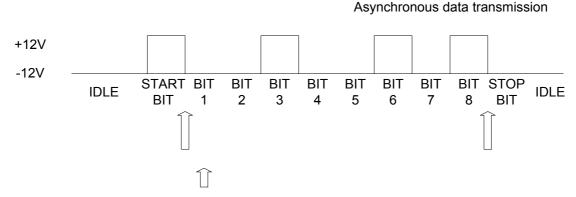
Receiver samples in middle of each data element
