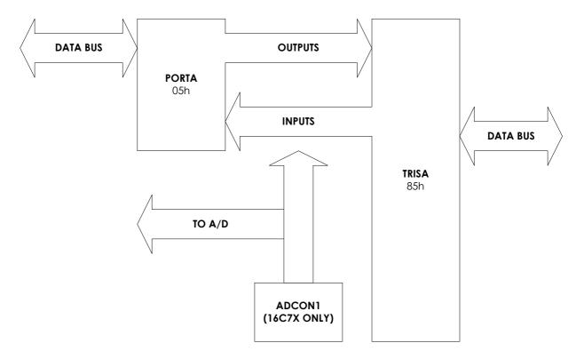
Port A has 5 or 6 lines – depending on the PIC – which can be configured as either inputs or outputs. Configuration of the port direction is via the TRISA register. Inputs are set with a 1 and outputs are set with a 0. The pins have both source and sink capability of typically 25mA per pin.
