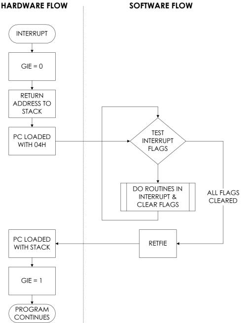
The hardware is completely under PICmicro® MCU control, the software is all your responsibility. When an interrupt occurs, the first step is to test and determine if the source is the desired one or, in the case of multiple interrupts, which one to handle first, etc.
