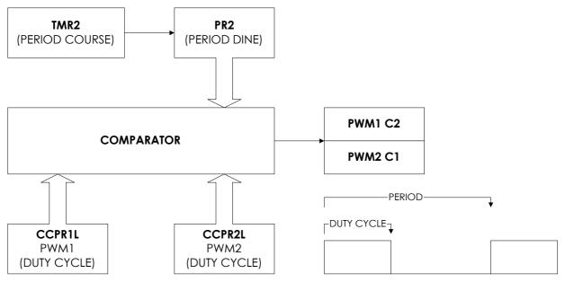
For PICmicro<sup>®</sup> MCU's with PWM generation hardware, once the registers are set up, the PWM runs on its own without constant software involvement. Calculation of the PWM values is best achieved with a simple spreadsheet. Example:
