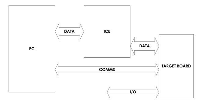
Using such a layout enables basic I/O and comms to be evaluated, tested and debugged. The use of the ICE, through not essential, speeds up the development costs and engineer's headaches. The initial investment may appear excessive when facing the start of a project, but time saved in developing and debugging is soon outstripped.
