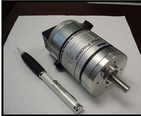
Figure 3.9 Litton - Clifton Precision Servo DC Motor JDH-2250
