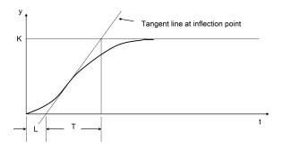
The S-shaped reaction curve can be characterized by two constants, delay time L and time constant T, which are determined by drawing a tangent line at the inflection point of the curve and finding the intersections of the tangent line with the time axis and the steady-state level line.
