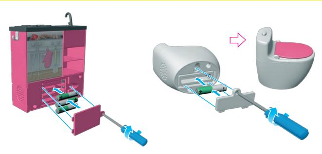
BATTERY INSTALLATION: Use a Phillips head screwdriver (not included) to open battery door. Insert 4 AAA batteries (not included). Replace battery door and tighten screws. Dispose of batteries safely. Replace batteries when sounds become garbled or faint or light dims. For longer life, use only alkaline batteries. When exposed to an electrostatic source, the product may malfunction. To resume normal operation, remove and re-install the batteries.
