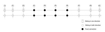
Figure 8. Eyiste Viaduct modified bearing conditions
