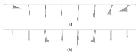
Figure 12. Eyiste Viaduct pier moment diagrams due to uniform temperature change (a. initial design; b. modified model)
