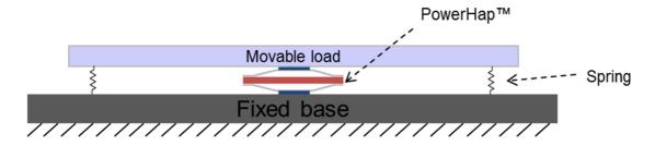
By applying a voltage to the actuator, it elongates and therefore moves the load. This movement can be felt by the user. For a maximal haptic feedback, the rear panel needs to be as heavy as possible. Otherwise the PowerHap<sup>™</sup> actuator will not only move the load but also the rear panel and therefore a part of the performance is lost.
