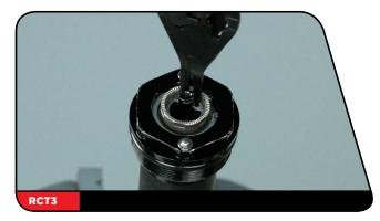
**RC Only:** Use small snap ring pliers to remove the retaining ring from the bleed plug.
