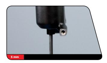
**5** Place an oil pan beneath the fork to catch any draining fluid.
