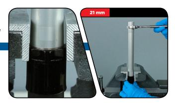
**RCT3 Only:** Use small snap ring pliers to remove the retaining ring from the low speed compression adjuster.
