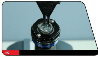
**RCT3 Only:** Use needle-nose pliers to remove the low speed compression adjuster from the compression top cap assembly.
