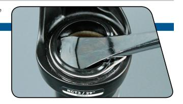
Stabilize the lower legs on a bench top or on the floor. Press down on the tire lever handle to remove the dust wiper seal. Repeat on the other side.
