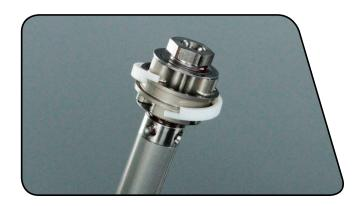
2 Clamp the wrench flats of the Charger Damper™ coupler into a vice. Place a 21 mm open wrench on the wrench flats of the cartridge tube. Hold the bladder assembly in place and turn the wrench counter-clockwise to loosen and remove the cartridge tube from the coupler. Pour the suspension fluid into an oil pan.
