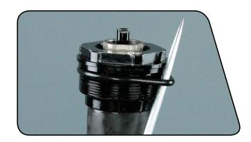
4 Lightly clamp the damper assembly into a bike stand with the rebound shaft facing up.
