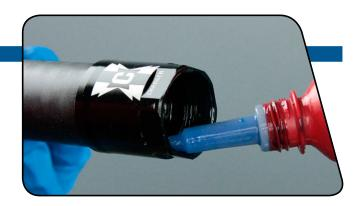
70 Thread the bladder assembly onto the cartridge tube assembly by hand.
