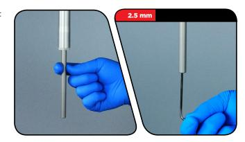
Fill the bleed syringe half full with 3wt suspension fluid and thread Fill the bleed syringe nail run with own same the syringe into the compression top cap assembly.
