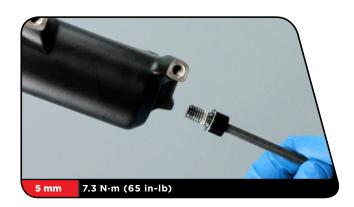
8 Install the rebound adjuster knob onto the rebound damper bottom bolt.
