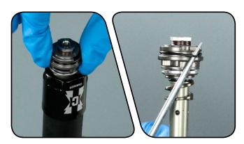
Clamp a 5/8" bit socket into a vise. Set the bladder assembly on the bit socket, and use a 25 mm open end wrench to remove the coupler.
