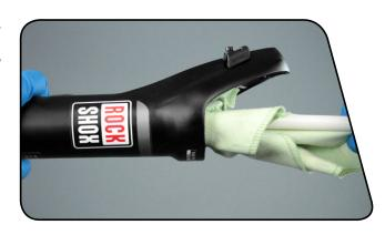
Reinstall new foam rings on the top bushings in the lower legs.
