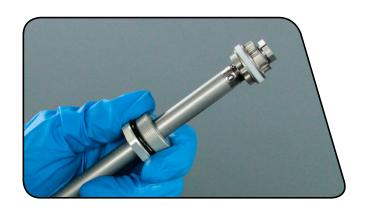
Use a pick or your fingers to remove the seal head o-ring. Use a pick to pierce and remove the scraper.
