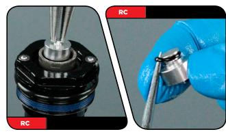
**RCT3 Only:** Use small snap ring pliers to remove the retaining ring from the compression cam assembly.
