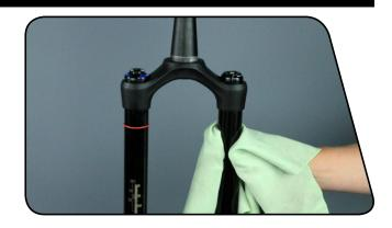
Apply a liberal amount of suspension specific grease to the inner surfaces of the dust wiper seals.
