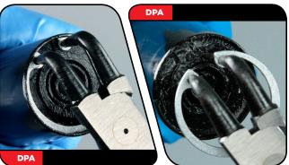
**Solo Air Only:** Use a flat head screw driver to push the SA seal head tab under the retaining ring.
