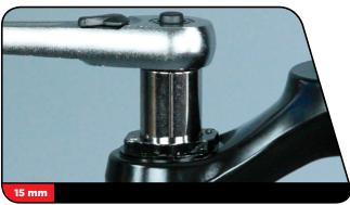
**RCT3 Only:** Place the compression mode adjuster knob onto the Charger Damper™ assembly with the long tab near the **front** of the crown. Turn the compression mode adjuster **clockwise** until it engages the first detent space.
