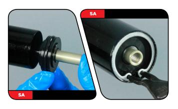
Insert the top cap into the top of the upper tube. Use a torque wrench with a 24 mm socket to tighten the top cap to 28 N·m (250 in-lb).
