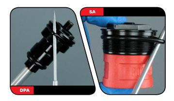
**Dual Position Air Only:** Push the air shaft into the upper tube to prevent scratching the air shaft when removing the retaining ring. Scratches on the air shaft will allow air to bypass the seal head into the lower legs, resulting in reduced spring performance.
