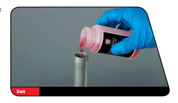
Use the palm of your hand or a rag to cover the cartridge tube, and cycle the rebound assembly shaft a few times to help pre-bleed air from the damper.
