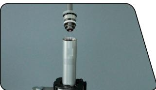
Remove the damper assembly from the bicycle stand and pour the suspension fluid into an oil pan.
