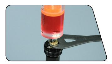
Hold the rebound shaft in place and pull up on the syringe handle to create a vacuum in the bladder.
