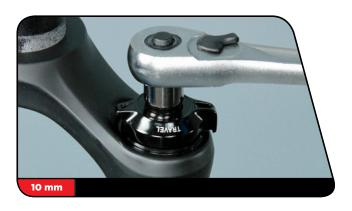
Use a 24 mm socket wrench to remove the top cap.
