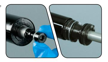
**Z** Spray isopropyl alcohol on the inside and outside of the upper tube. Wipe the outside of the upper tube with a clean rag.
