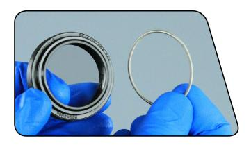
Insert the narrow end of a new dust wiper seal into the recessed end of the seal installation tool.
