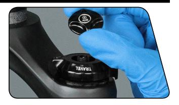
Use a small hex wrench to depress the Schrader valve and release all of the air pressure from the air chamber.
