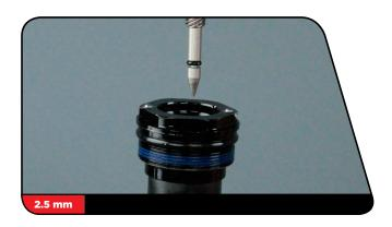
**RCT3 Only:** Insert the compression cam assembly into the bladder assembly and turn clockwise to lock into place.
