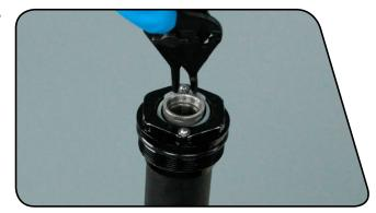
Open the rebound assembly by pulling down on the rebound shaft to extend it. Then insert a 2.5 mm hex wrench into the bottom of the rebound shaft and turn it counter-clockwise until it stops.
