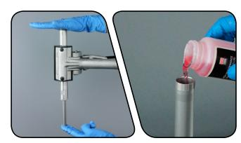
Wrap a rag around the cartridge tube. Insert the compression piston assembly into the cartridge tube.
