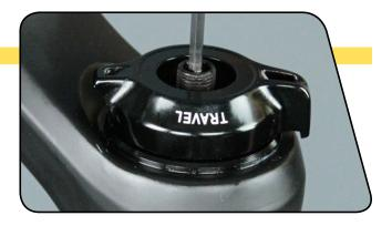
**Dual Position Air Only**: Use a 10 mm socket wrench to loosen and remove the DPA Adjuster Knob.
