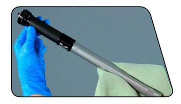
Insert and thread the compression top cap assembly into the top of the upper tube. Use a torque wrench with a 30 mm socket to tighten the compression top cap assembly to 28 N•m (250 in-lb).
