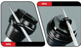
**Solo Air Only**: Use a pick or your fingers to remove the air piston quad ring.
