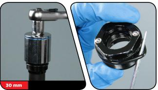
Turn the bladder assembly over to remove the compression piston assembly.
