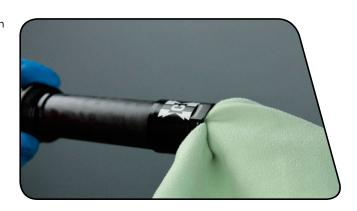
9 Apply a small amount of Loctite® Threadlocker Blue 242® to the coupler threads.
