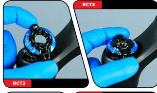
**RC Only:** Place the compression mode adjuster knob onto the Charger Damper assembly with the long tab near the **back** of the crown. Turn the compression mode adjuster **counter-clockwise** until it engages the first detent space.
