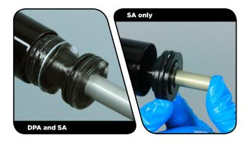
**Dual Position Air Only:** Push the air shaft into the upper tube to prevent scratching the air shaft when installing the retaining ring.
