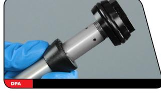
**Solo Air Only:** Install a new bumper cone with the broad base facing away from the SA piston.
