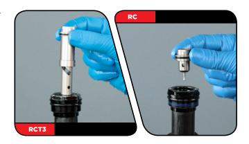
RCT3 Only: Use snap ring pliers to install the outer retaining ring to secure the compression cam assembly. Use a rag to soak up excess fluid.
