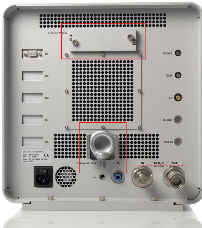
Figure 8. The transport hook and the fixation pieces are stored at the back of the detector
