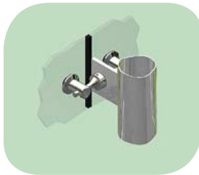
Pilkington Planar ™ 905J fitting to a tubular steel support structure.
