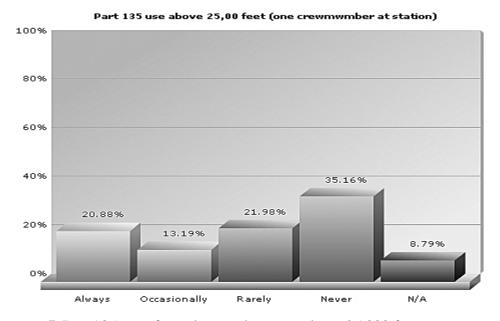
Figure 7. Part 135 use of supplemental oxygen above 25,000 feet.
