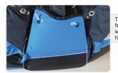
The container can be closed by running both zips forward towards the reserve parachute opening, all the way to the eyelets, and then back again underneath the harness to secure the zips
