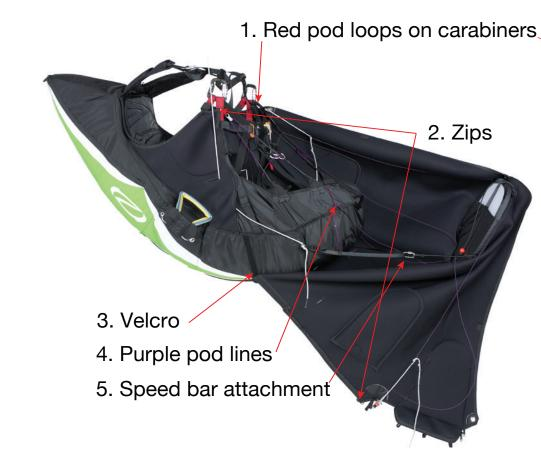
IMPORTANT: Ensure the red pod loops (1) are attached to the carabiners. Failure to do so will put excessive load through the zip causing failure.
