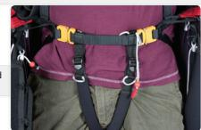
Fasten the leg/chest strap with the orange buckles. Ensure that the buckles are closed properly and that both the upper and lower buttons click into place.
