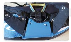
Gently pull the parachute handle and top flap out of the way so they are clear of the bottom flaps
