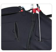
Then pass the line through the Ronstan pulley, ensuring that the pulley is not twisted before routing the line through the small gap into the pod compartment.
