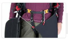
The automatic pod closing system should now be connected. First attach the red loop of the left hand pod flap to the red ball situated under the maillon on the right hand side of the harness. The red ball goes through the red loop.
