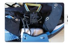
Pay attention to the bridles. Do not allow them to become entangled, they should remain neatly in place to the left hand side of the parachute when inserting.
