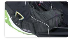
Ensure that the lines run cleanly between the pulleys and pass on the outside of all structural webbing straps. Double-check the lines have not inadvertently wrapped around any of the structural webbing straps. Attach the speed bar with a Bowline knot and repeat the procedure on the other side.
