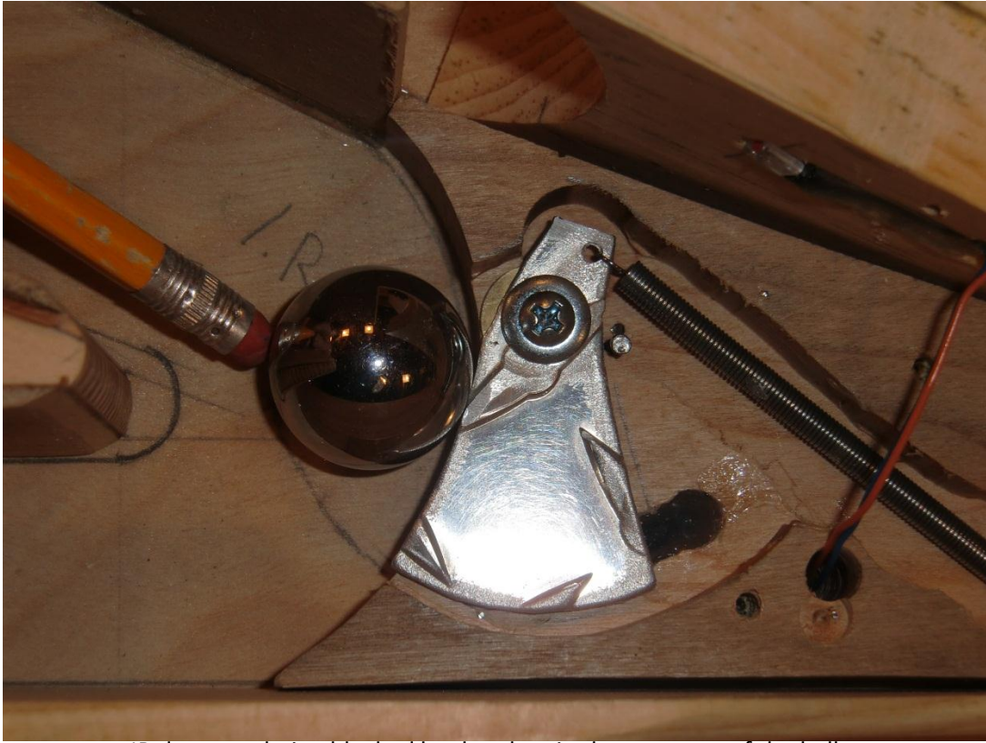
IR detector, being blocked by the plate in the presence of the ball
