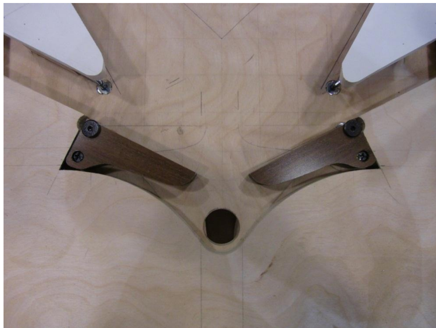
Flipper, cross nut below, axial bolt above.
