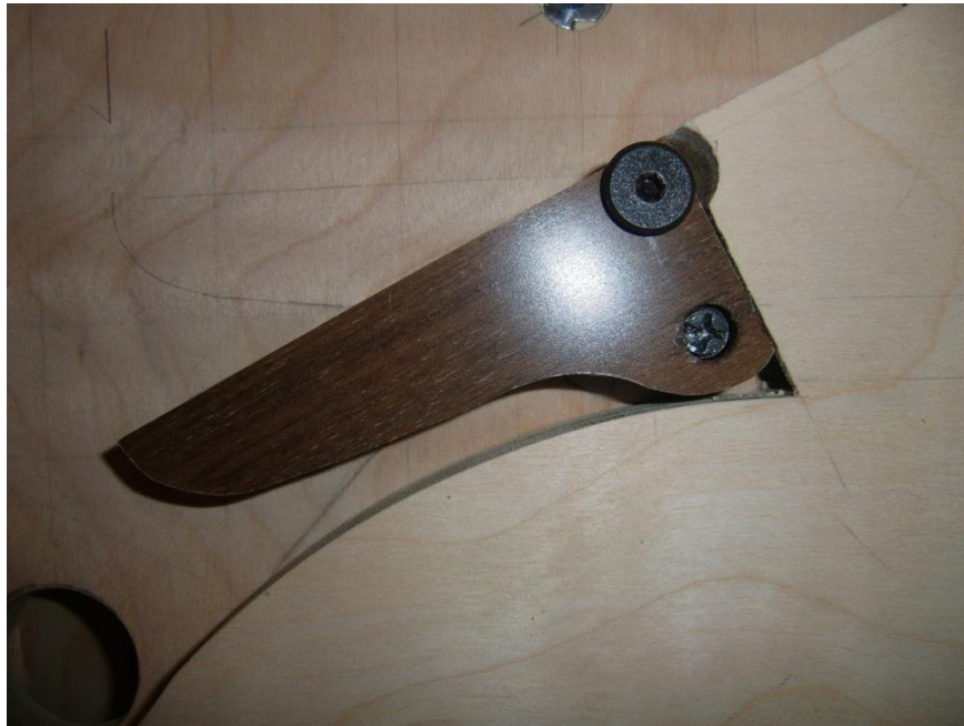
Flipper, cross nut below, axial bolt above.
