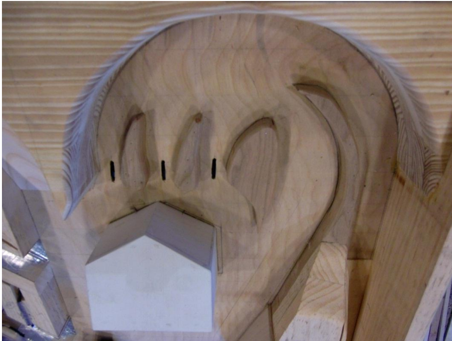
Three channels for the ball to enter at the top of the deck. (launch channel at far right)
