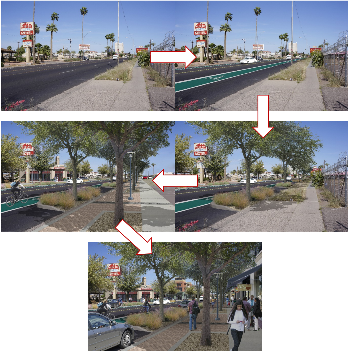
Image 14: A street conversion from traffic circulator to fully integrated street in several manageable phases. Source: Duany Plater-Zyberk & Co.
