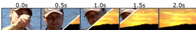
Here is the same transition as above, this time using actual video. For clarity, the transition boundary in the three center frames has been emphasized in white. Both clips continue to run while the transition is in progress.
