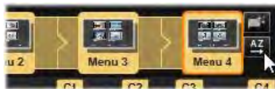
Pages from a multipage menu. The connector graphic shows that navigation within these pages is provided by Next and Previous buttons. The Sort button (top right, under pointer) arranges the chapter buttons in timeline sequence.
