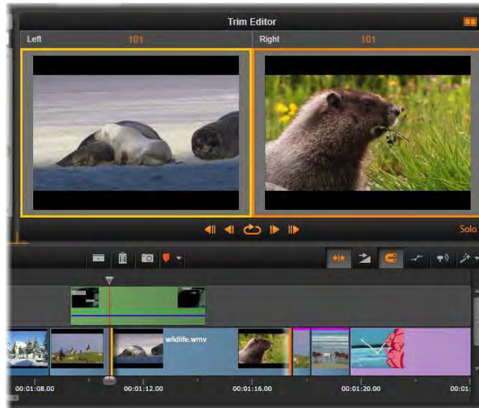
The Trim Editor in a slip trim operation. The left preview shows the currently selected trim point; the right preview shows the second trim point.
