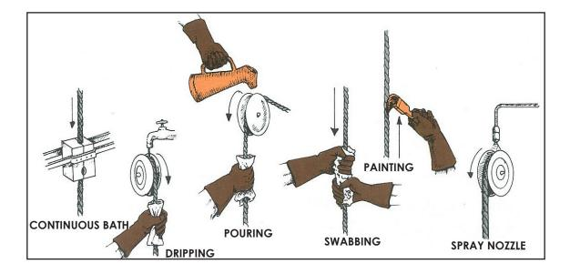
The illustrations above are proper methods of appling lubrication to a rope in service. The arrows indicate the direction of the ropes' movement.
