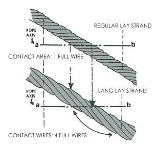
The above is a comparison of wear characteristics between regular lay and lang lay ropes. The greater metal area along the rope's axis (a-b) promotes more wear-resistance than a regular lay rope. The longer exposed length of outer wires in a lang lay rope offers an easier bend, resulting in greater fatigue resistance (page 9).
