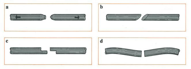
A wire broken under a tensile load that exceeds its strength is recognized by the "cup and cone" configuration at the fracture point (a). The *necking down* of the wire at this point shows that failure occurred while the wire retained its ductility. Shear-tensile fracture (b) occurs in wire subjected to a combination of transverse and axial loads. Fatigue breaks are usually characterized by squared-off ends perpendicular to the wire either straight across or Z-shaped (c & d).
