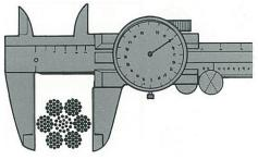
The true diameter of wire rope is measured at it's largest point.
