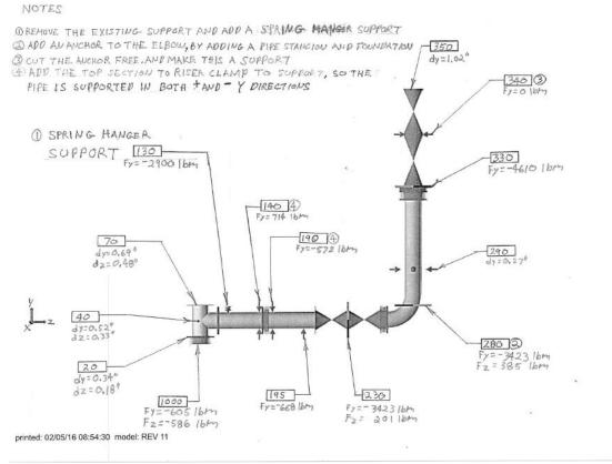
Figure 2: Analysis of an engine exhaust system under hot conditions.
