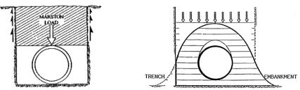
Figure 1a, b: Marston Load (ASCE 2009), and Soil Arching (Watkins 2001)
