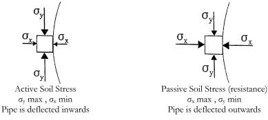
Figures 4a, b: Active and Passive Soil Stresses
