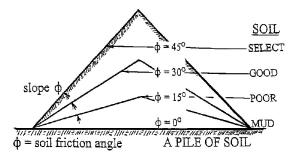
Figure 2: Soil Friction Angle,  $\varphi$ , for Various Soil Types
