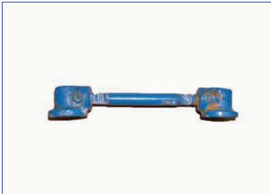
BlueCoat treated single pipe roll support after 2500 hours.
