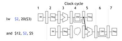
Notice that we're still using forwarding in cycle 5, to get data from the MEM/WB pipeline register to the ALU
