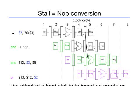
The effect of a load stall is to insert an empty or nop instruction into the pipeline
