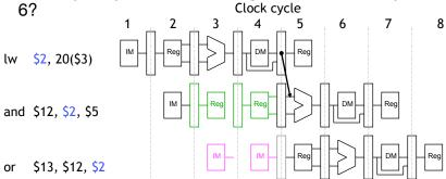
Those units aren't used in those cycles because of the stall, so we can set the EX, MEM and WB control signals to all 0s ... the bubble "bubbles" through
