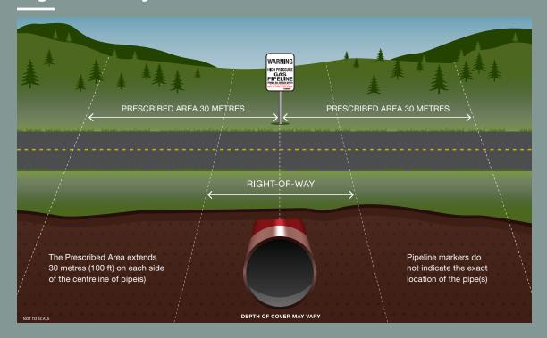
A pipeline right-of-way (ROW) is the strip of land where the pipeline is located. The width of the ROW may vary depending on factors such as pipeline diameter or the number of pipelines in an area. The area extending 30 meters (100 feet) on either side of the pipeline is called the Prescribed Area / Controlled Area.
