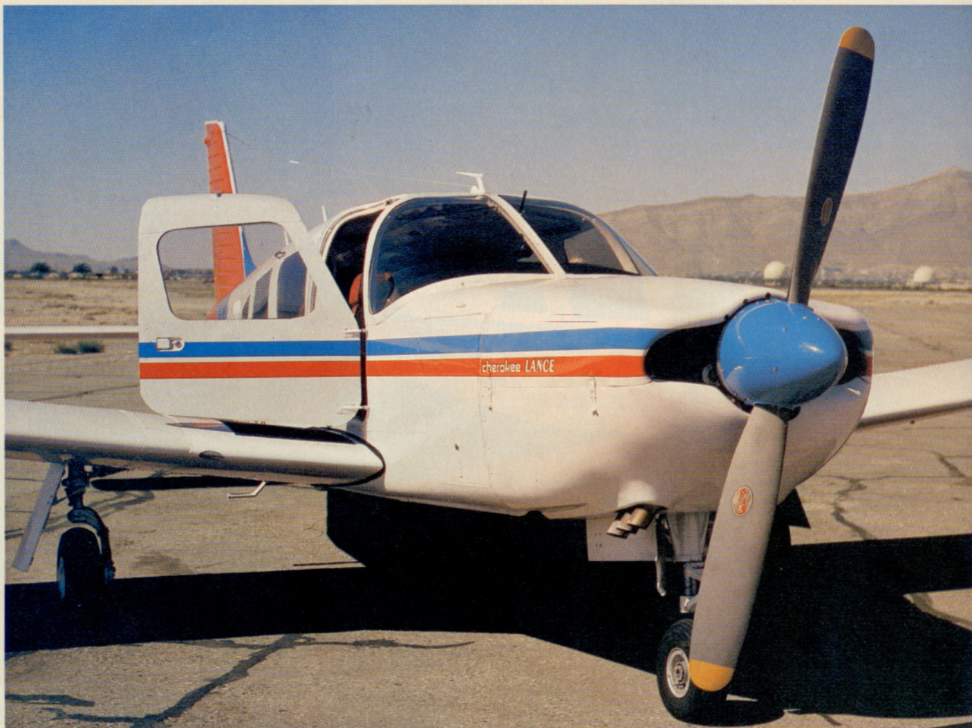
The Lance's new gear gives the aircraft a near-level stance, aiding taxiing visibility and ridding the Lance of the Cherokee Six's snout-high silhouette. Photos by the author except as noted.
