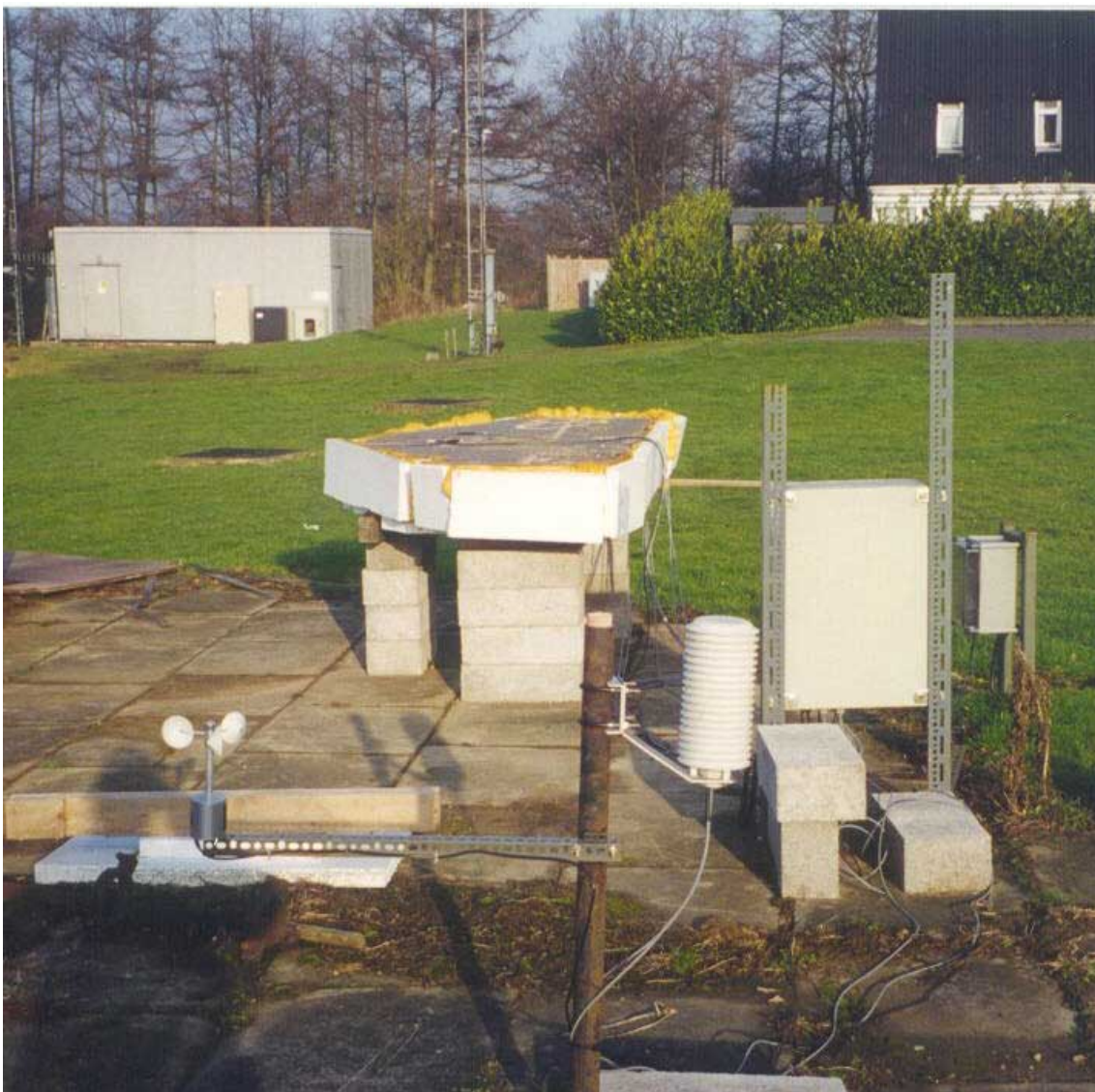
Figure 9.2.4 - 6 Slab S2 exposed at BRE for temperature recording
