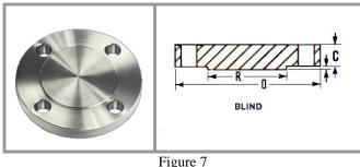
While the Blind flange is used to cap off the end of a pipeline or a future branch connection it is also used for other purposes. It can be drilled and tapped for a threaded reducing flange or machined out for a Slip-On reducing flange. The reduced opening can be either on-center or eccentric.
