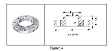
The Lap Joint flange requires a companion lap joint, or Type A stub-end (ref. Fig. 5) to complete the joint. The installer is then able to rotate the flange. This allows for quick bolthole alignment of the mating flange during installation without taking the extra precautions required during prefabrication of a welded flange.
