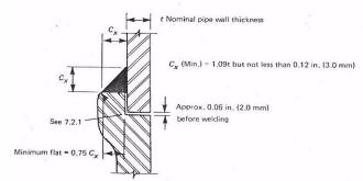
Figure 10 – Socket Weld Fitting Joint from ASME B16.11
