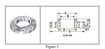
Unlike the Socketweld flange, the Slip-On flange allows the pipe to be inserted completely through its hub opening. Two welds are made to secure the flange to the pipe. One fillet (pronounced "fill-it") weld is made at the hub of the flange and a second weld is made at the inside diameter of the flange near the flange face.
