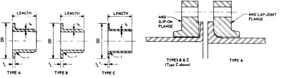
Type C (Fig 5) is fabricated from pipe using five suggested methods indicated in ASME B31.3. The most prevalent of these is the machine flare. This is done by placing a section of pipe into a flaring machine, flaring the end of the pipe and then cutting it to length.
