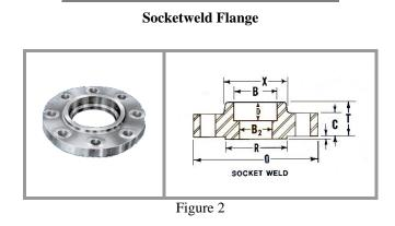
The Socketweld flange is made so that the pipe is inserted into the socket of the flange until it hits the shoulder of the socket. The Pipe is then backed away from the shoulder approximately 1/16" before being welded to the flange hub.
