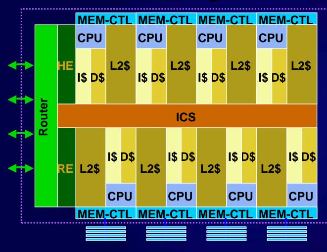
Alpha core: 1-issue, in-order, 500MHz L1 caches: I&D, 64KB, 2-way Intra-chip switch (ICS) 32GB/sec, 1-cycle delay L2 cache: shared, 1MB, 8-way Memory Controller (MC) RDRAM, 12.8GB/sec Protocol Engines (HE & RE): μprog., 1K μinstr., even/odd interleaving System Interconnect: 4-port Xbar router topology independent 32GB/sec total bandwidth
