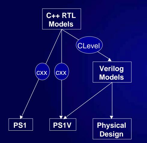
cxx: C++ compiler CLevel: C++-to-Verilog Translator **C++ RTL Models:** Cycle accurate and "synthesizeable"
