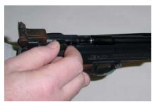
**Step 3.** With the pistol pointed in a safe direction, extend cocking lever/handle fully until air is sucked in, pause 2 seconds, and close the handle until it is locked back in place.
