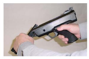
**Step 3.** With the muzzle pointed in a safe direction, "break" the barrel and bend until spring "clicks" in place.
