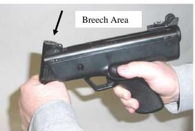
**Step 5.** Firmly grip the muzzle end and pistol grip and "snap" barrel back into place.
