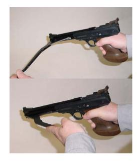
Multi-pumps will take several additional pumps of the cocking lever to charge the amount of pressure needed for the shot.
