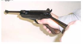
**Step 4.** Place pellet into the breech area of barrel making sure to press the pellet in flush to the edge of the barrel. The flat head of the pellet should be toward the muzzle and the skirt end toward the rear.
