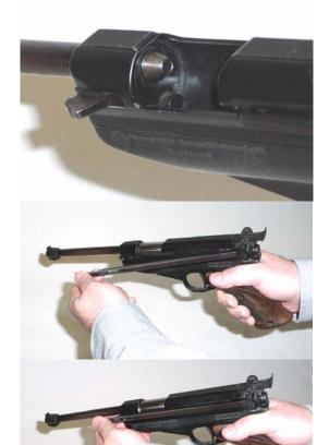
**Step 5.** Fold lever back and clip in place.
