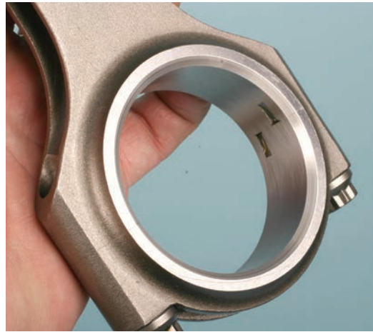
If a large chamfer is present as shown here, this side of the rod faces the radius fillet of the crank journal.
