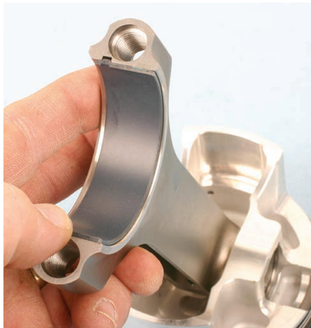
Bearing tangs register to the tang grooves in the rod and cap simply to provide a locating aid to place the bearings in the correct fore-aft position, to eliminate potential mistakes in bearing location. Bearing crush that results from cap tightening serves to lock the bearings in place to prevent bearing spin. Note how this bearing is registered slightly biased away from the chamfered side to prevent the bearing from digging into the crank fillet.
