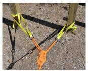
This anchor point demonstrates the concept of load sharing by attaching several deck posts to anchor webbings clipped into a single, split looped Super 8 knot.
