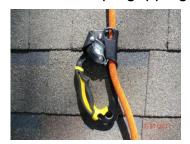
**WARNING:** Ascenders can fail with as little as 600 lbs of load force therefore are not approved by manufacturers to use alone as a primary belay device! **Petzl Chest Ascender** (Croll) – (Aluminum) Tensile breaking strength = 1,240 lbs. when attached to 10.5 mm rope. Chest positioned rope gripping device used to ascend a lifeline. Retirement at 10 years or sooner based on condition.
