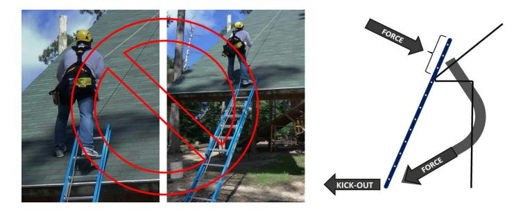
**Ladder Kick-Out** – is the leading cause of ladder access related injuries that occurs when the dynamic forces applied to the ladder exceed the traction of the ladder's base footing. The application of climber's weight to any rung located above the rail contact points at the eave of the roof can cause catastrophic ladder failure.
