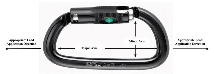
**Warning:** Carabiners represent a quick and easy way of establishing a rope access connection however, to avoid compromising a carabiner's greatest listed strength, they should always be loaded in a single direction along the major access with the gate securely closed.
