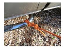
**Examples of Appropriate Fixed Anchors:** Trees, fence posts, deck posts, heavy shrubs, fire hydrants, anchor barrels and vehicles.
