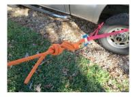
Establishing an anchor point around an axle or tire rim is an effective means of securing a lifeline however, should incorporate the use of tubular webbing to prevent shear damage to a rope.
