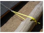
• **Anchor Slings** – Heavy duty braided nylon of varying lengths with stitched looped ends used to expedite the set-up of an anchor connection point. Tensile breaking strength: End to End = 9,000 lbs., Basket loop = 18,000 lbs.
